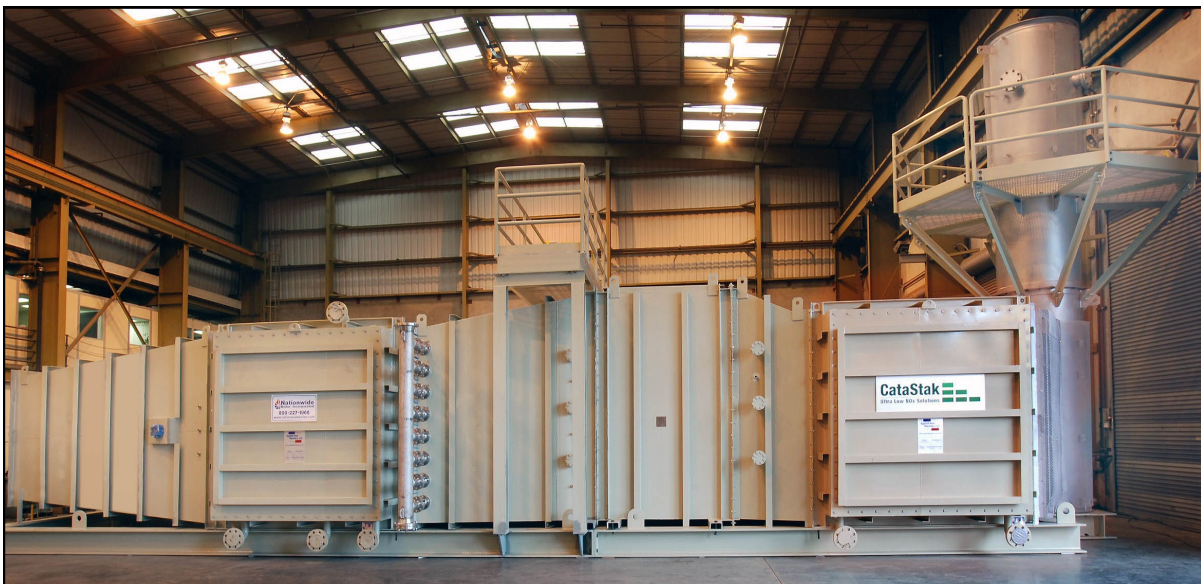
Pictured at top: Solar Saturn compressor set with duct waste heat recovery operating at 2½ ppm NOx (@15% O2). Pictured at bottom: Complete CataStak™-GT SCR system including HRSG and duct burner ready for shipment at Nationwide Boiler's shop.
